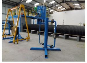
Confined Spaces, a complex 30 metre multi directional confined space training facility has been constructed combining vertical and horizontal chambers along with the mock refinery distillation column used to train workers in both safe working practices and rescue procedures.
